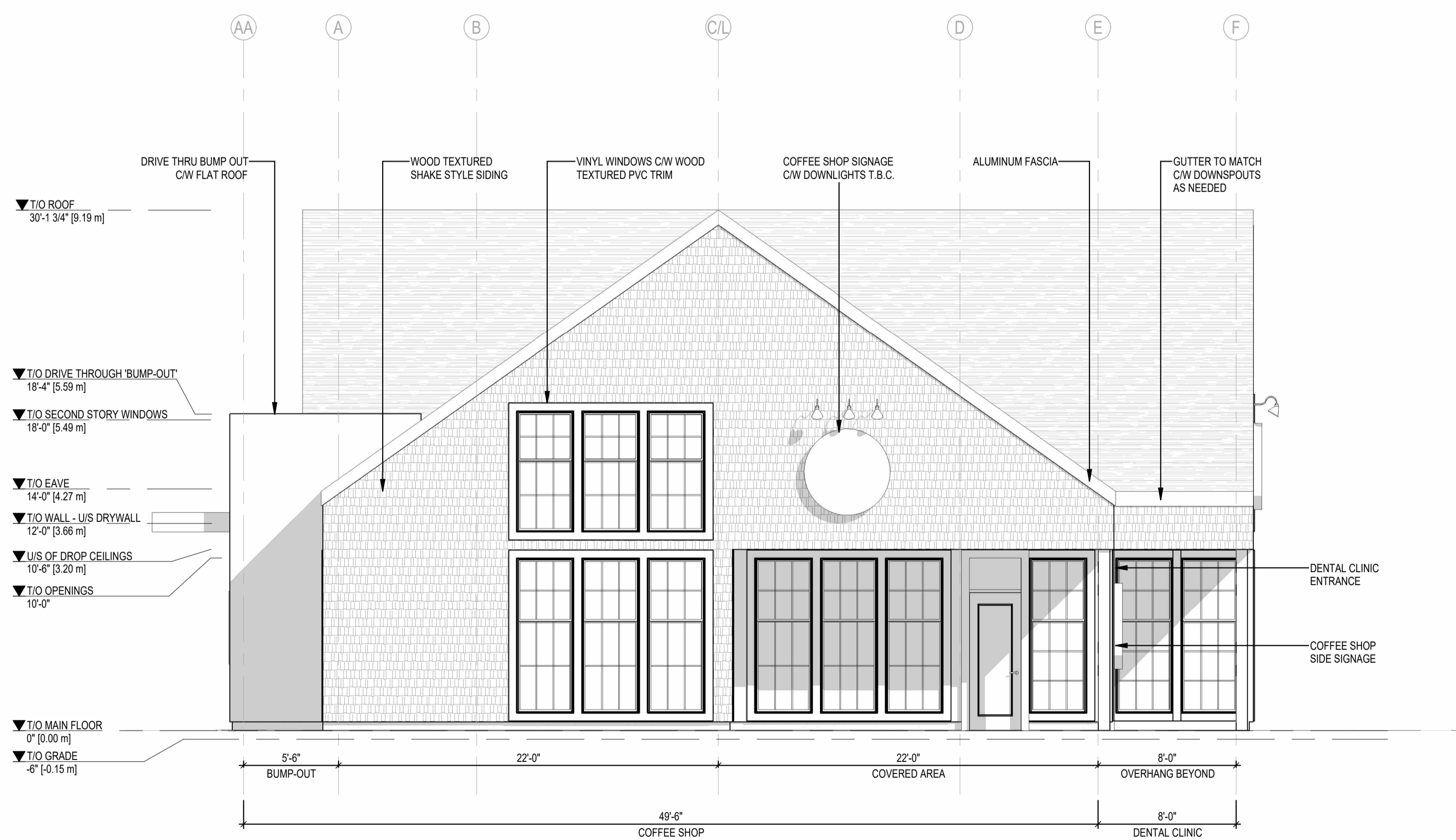
2 WEST ELEVATION SCALE: 3/16" = 1'-0"
